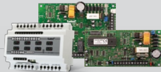
expansion zones and outputs modules
